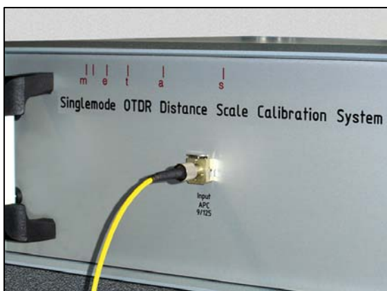
Fig. 3. Multi-purpose Adapter System (MAS) interface on instrument front panel.
