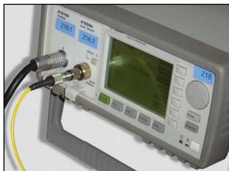
Fig. 2. UGT as sacrificial interface on instrument front panel.
