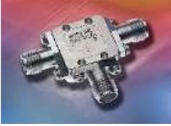
MITEQ is offering a new line of mixers designed specifically for Satellite applications. The TBS2731LW1 is ideally suited for converting from L-band to Ka-band or Ka-band to L-band. The mixer has superb conversion loss and VSWRs as well as excellent spurious response and outstanding LO isolations. This device meets rugged environmental MIL specs, operates over a  $-54$  to  $+85^{\circ}\text{C}$  temperature range and is ideal for rugged Military and Commercial system applications.
