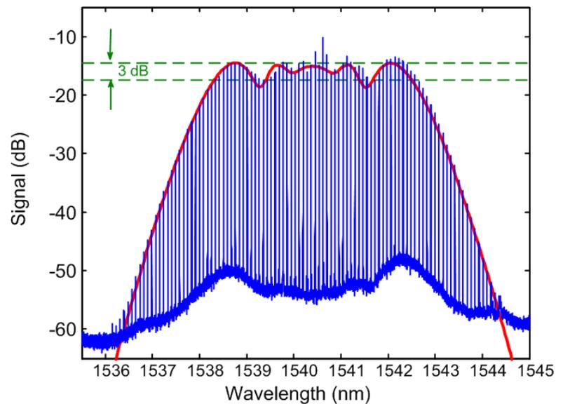
Figure 8: Optical spectrum of expanded Pilot Photonics' OFCS measured by APEX UHR-OSA, by fiber nonlinearities based expansion techniques
