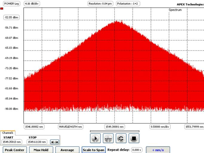
Figure 1: Pritel's OFCS spectrum measured by APEX-UHR-OSA with 5 MHz/0.04pm frequency resolution, the pulse repetition frequency is around 20 MHz.
